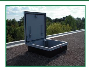
**Note:** For Stainess Steel Roof Hatch, should the cover show black stains due to melting of the protection plastic, remove stain by using an abrasive paper (4000 or 6000 or Green scrub pads) and sand in the grain direction.
