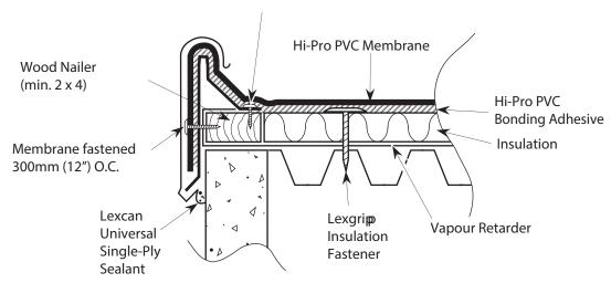
Comments: Fasteners must embed into nailer 25mm (1") min.
