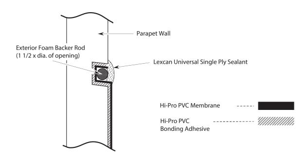
Comments: All membrane flashing must be a minimum of 200mm (8") above roof level.
