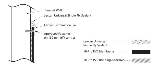
Comments: Flashing a min. 200mm (8") high whenever possible and must be above flood level.
