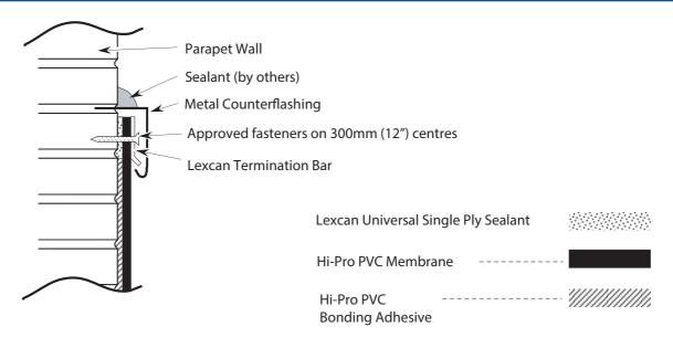
Comments: All flashing must be a minimum of 200mm (8") above roof level.
