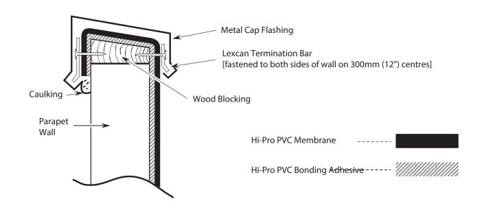
Comments: Masonry surfaces must be fully cured (min. 28 days) to facilitate proper bonding.
