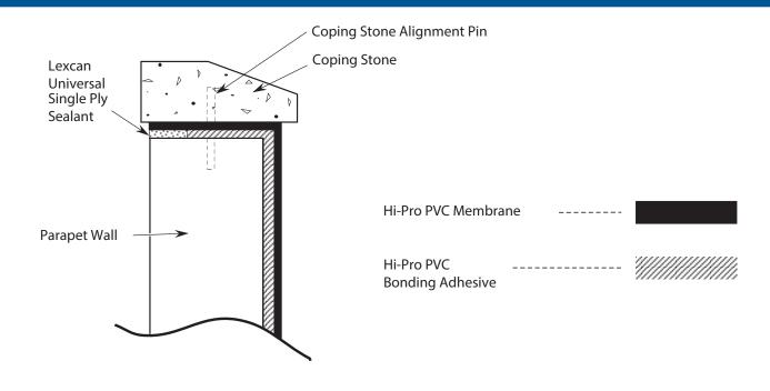
Comments: Masonry surfaces must be fully cured (min. 28 days) to facilitate proper bonding.
