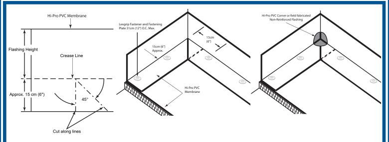
Notes: 1. Perimeter membrane fastening should be started within 15cm (6") of corner.
