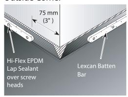
Fasten Lexcan Batten Bar to outside corner with Lexgrip™ Fasteners on 15 cm (6") centres .
