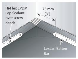
Fasten Lexcan Batten Bar to inside corner with Lexgrip™ Fasteners on 15 cm (6") centres.
