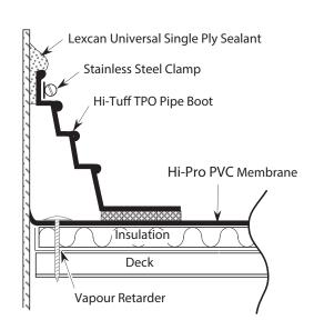
Comments: Scrub membrane and pipe boot with Lexcan Weathered Membrane Cleaner prior to welding.
